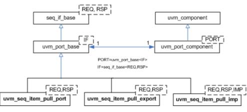
Sequencers and drivers use a *seq\_item\_port* specifically supports sequencer-driver communication. Connections to these ports are made in the same fashion as the TLM ports.
